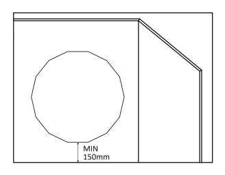
Sensor needs to be a minimum 150 mm away for any surface
