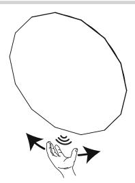
Your mirror comes with an infrared sensor located in the middie of the bottom. To activate the light and demisting pad, move your hand across the sensor once at a distance of around 5cm o turn it off, move your hand across the sensor again.
